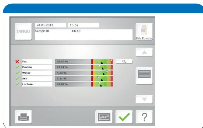
Figure 4: Result screen for a quantification showing a Mahalanobis outlier for the fat evaluation.
